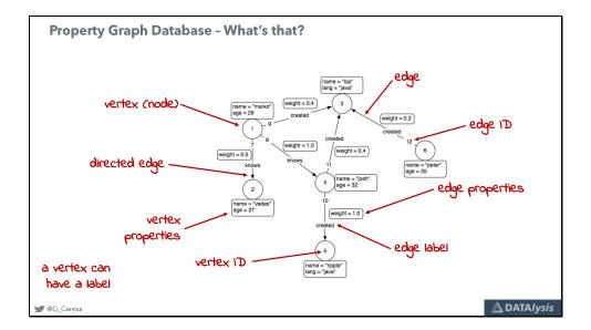
This is a visualization of an example graph: the 2 components, nodes and edges, are clearly visible.
