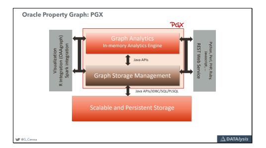
In Oracle the graph "engine", the brain, is called PGX. It's the acronym for Parallel Graph Analytics. PGX doesn't implement a full storage layer, it instead use existing options which could be an Oracle Database, an Oracle NoSQL database or HBase. Even a simple file in the filesystem.
