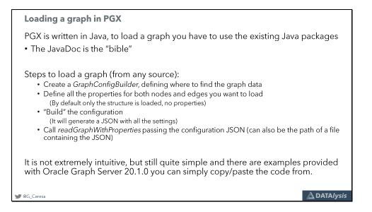
The process to load a graph in PGX is mainly creating a configuration defining where the graph is stored. Define which properties you want to load. Build the configuration which simply takes all the settings and some defaults to generate a Json string. And finally you can load the graph by using that Json (or a path pointing to a file containing the Json).
