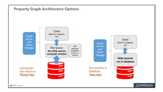
Oracle Property Graph can be used in 2 ways: the two tier approach which run graph queries directly on the Oracle database used for storing the graph. The graph query language, PGQL, is translated into standard SQL to provide the answer to the request.
