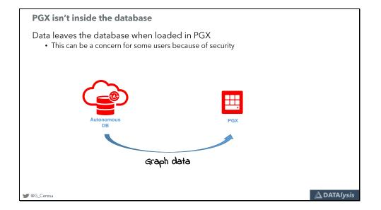
PGX, the "engine" powering property graph in Oracle, is a separate process than the database. This means that when a graph is loaded in PGX, the data is leaving the database to be loaded into PGX:
